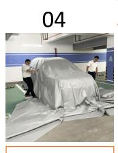
Quickly use your feet to step firmly around the car fire blanket.
